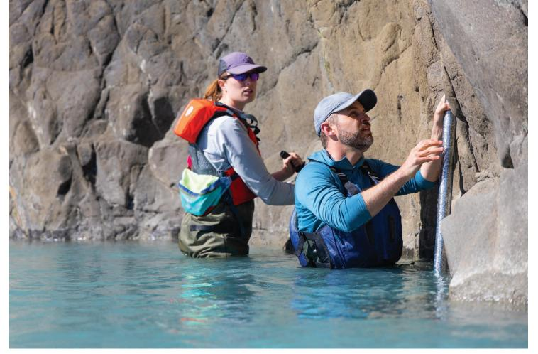
**ABOVE**: Camryn Kluetmeier and Tamlin Pavelsky install a waterlevel logger in the Waimakariri River. RIGHT: Marissa Dudek collects GPS coordinates for a GNSS survey and documents times for a water-level logger installation.
