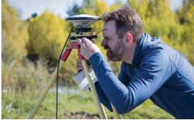
ABOVE: Tamlin Pavelsky is the freshwater science lead for the SWOT project. LEFT: Pavelsky attaches a global navigation satellite system (GNSS) receiver to an antenna on top of a tripod to collect GPS points from various satellites.
